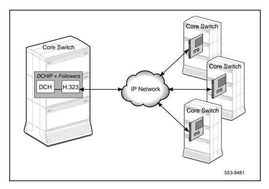
The ISL connection to the Meridian 1 functions as it does in a normal ISDN network. The ISL controls the call processing for calls over analog ITG IDSN Signaling Link (ISL) TIE trunks. These ISL TIE trunks can be on any of the ITG ISL Trunk cards. The ITG ISL D-channel only controls ITG ISL Trunk cards in the same ITG node. MAT administration relates the cards with trunks to the DCHIP ITG Trunk card.
